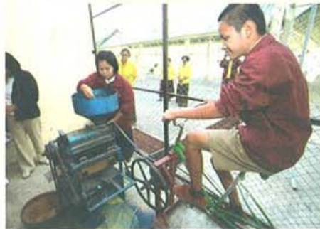
The school's pedal-powered grain mill.
